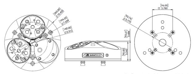
Note: The 95.76mm (3.77") diameter pattern is designed to fit both the 95mm and 3.8 inch pallet patterns utilized by the Matsuura MAM72-35V pallet.
